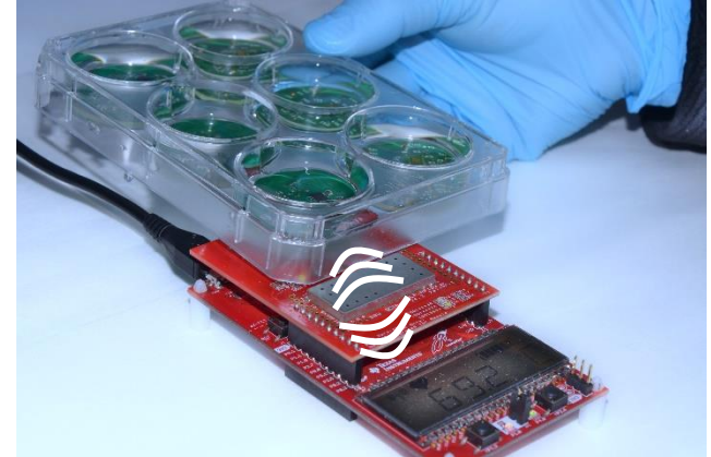
Test PCB platform comprising an RF communication block with antenna and temperature sensor
